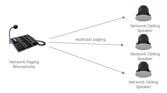
The Network Ceiling Speakerr GEN-6212A01 support Onvif protocol which can be registered to the 3-rd party monitoring system ,and during emergency situation ,the operator can directly make a live announcement to the speaker on the monitoring platform.
