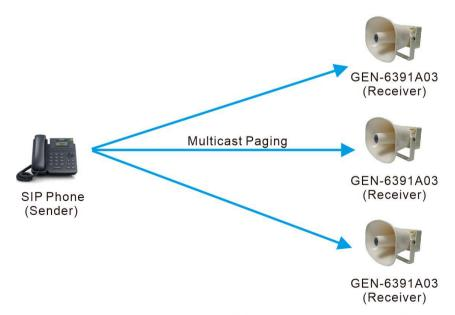
\*No SIP registration required for speakers in a multicast
